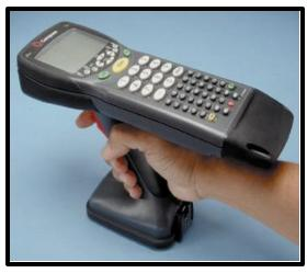
The *Apex IV* supports Batch or RF operations via an internal type III PC Card port (capable of simultaneously supporting two type I or II devices). This port provides the user with numerous options for connectivity and memory expansion including, but not limited to network interface adapters, high speed modems (both wired and wireless), Flash drives and RAM disks.
